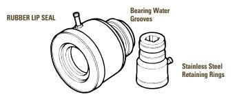
Another common type of mechanical seal used on rotating propeller shafting is the lip seal. Lip seals are similar to stuffing boxes in that they utilize the propeller shaft as a sealing surface. A rubber ring with a lip on the inside diameter fits over the propeller shaft. The tight interference fit between the rubber lip and the propeller shaft ensures continuous contact and creates a seal.
