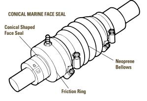
Conical marine face seals have a seal ring with a beveled face and a mating friction ring with a counter bevel. Any vibration or misalignment will cause the conical face to wear into an oval or elliptical shape. This prevents the seal from seating correctly, causing it to leak.
