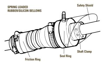
Any bellows-type seal uses the bellows as the only barrier between you and the sea. If the bellows should fail or be damaged, a serious leakage situation will occur.
